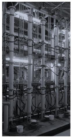
After the successful proof of concept, Phase 2 involves a 4,800kg sulphide bulk sample being used for a series of sulfation tests, irrigation acid consumption mini columns, 1m sequential columns and 4m columns.
